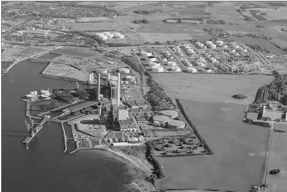
**Figure 11.3 Oil refinery in Kalundborg, Denmark.** *A collaboration – an industrial symbiosis – is pursued by the refinery with several other production companies in the Kalundborg area, which make commercial use of each other's spent coolant water and waste products. (Photo: TA Foto Scandex AS)*
